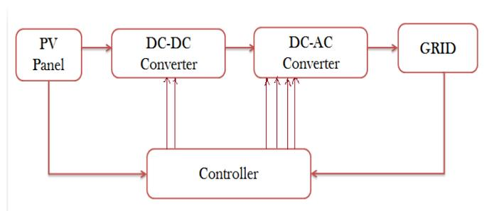
Fig 1: Block diagram of grid connected PV micro inverter
