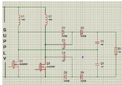
**Fig 4 :** Quadrupler circuit
