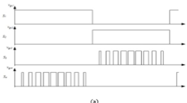
Fig: 3 The HPWM signals on the switches of the full-bridge inverter.
