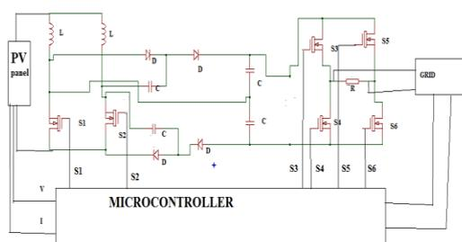
Fig.2. circuit diagram of micro inverter
